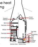
close to but completely separate from, the firing chamber. The gap between the two structures is about the width of a building brick. The freestanding firing chamber could be maintained, or even demolished and rebuilt,
